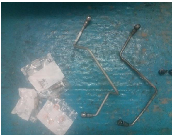
New oil feed pipe.
