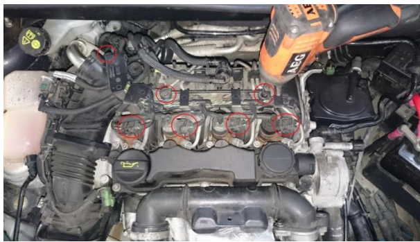
Disconnect wiring loom.
