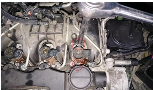
Remove 2x bolts, slide injector up.
