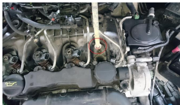
Make sure the copper washer comes out.
